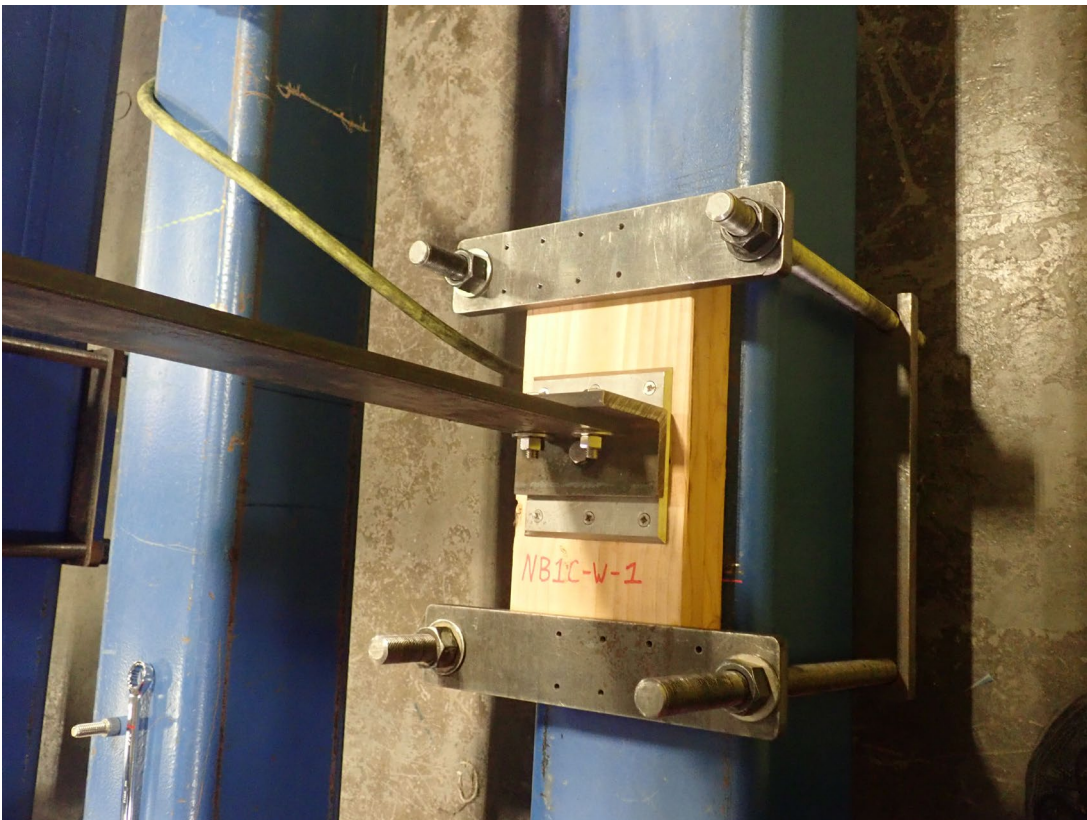
Photo 2 – File No. PA300986 Typical Test Setup with Steel 90° Angle
