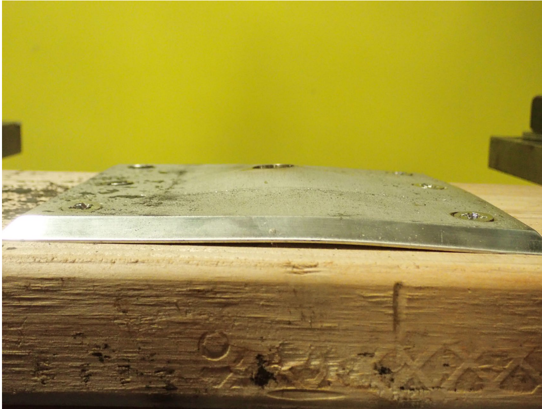
Photo 3 – File No. PA300990 Serial No. NB1C-W-3 Ultimate Test Deformation
